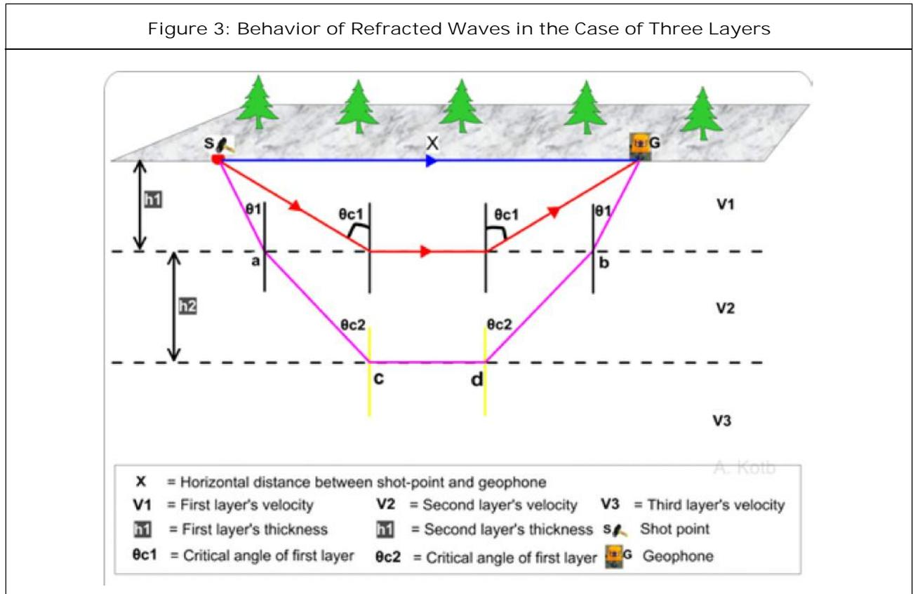
$$\frac{X_{d2}}{v_2} - \frac{X_{d2}}{v_3} = \frac{2h_1\sqrt{v_3^2 - v_1^2}}{v_3v_1} - \frac{2h_1\sqrt{v_2^2 - v_1^2}}{v_2v_1} + \frac{2h_2\sqrt{v_3^2 - v_2^2}}{v_3v_2} \quad \dots(15)$$
