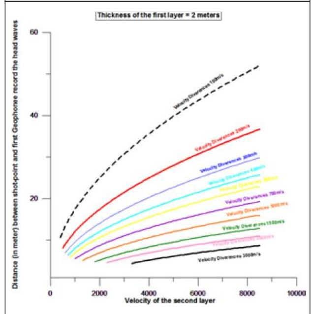
Figure 6: Main Relation Between (Velocities of First and Second Layers  $V_2/V_1$ ), and (First Layer's Thickness and Shortest Distance Between Shot-Point and First Geophone Which Can Record Head Waves  $X_{dn}/h_1$ )
